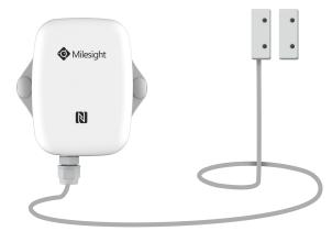
EM300-MCS is a compact magnet switch sensor for detecting open/close status of objects (such as doors or windows) and transmitting alarm using LoRaWAN® technology. With this low power consumption technology, EM300-MCS can work up to 5 years with 4000 mAh battery. Combining with Milesight LoRaWAN® gateway and Milesight IoT Cloud solution, users can manage all sensor data and remotely and visually and receive alarms via mobile App.
